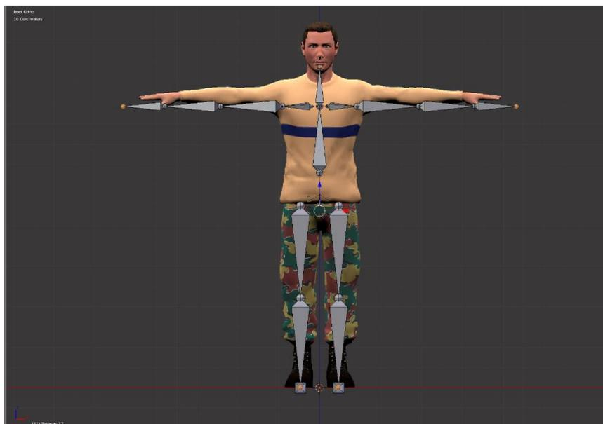
Fig.4.34 Armature from the motion tracking system half aligned with the mesh (front)
