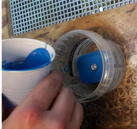
Fig.4.63 Pouring silicon to create an external mold
