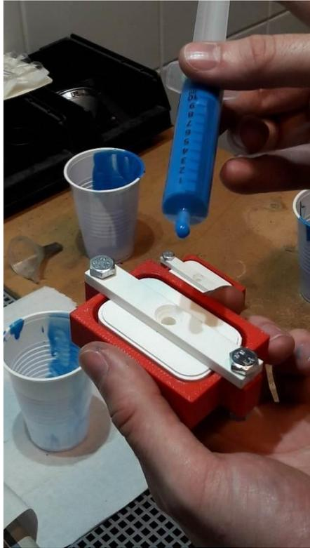
Fig.4.57 Pouring mold method
