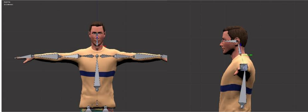
Fig.4.35 Armature from the motion tracking system aligned with the mesh (front and sagittal view)
