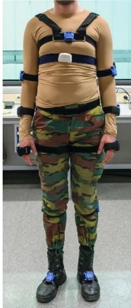
Fig.4.28 The subject wearing the smart shirt and the inertial system
