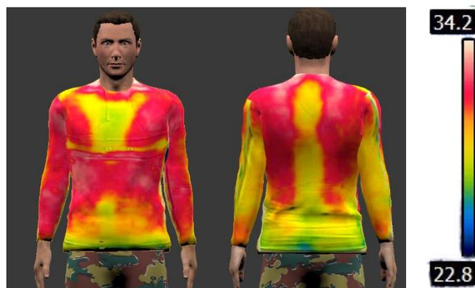
Fig.4.44 Thermophysiological evaluation in DHM on the first prototype after 30 minutes of exposure
