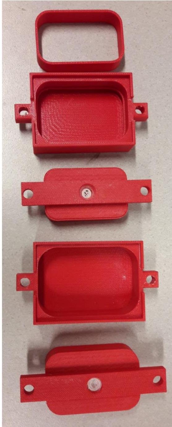
Fig.4.56 ABS mold
